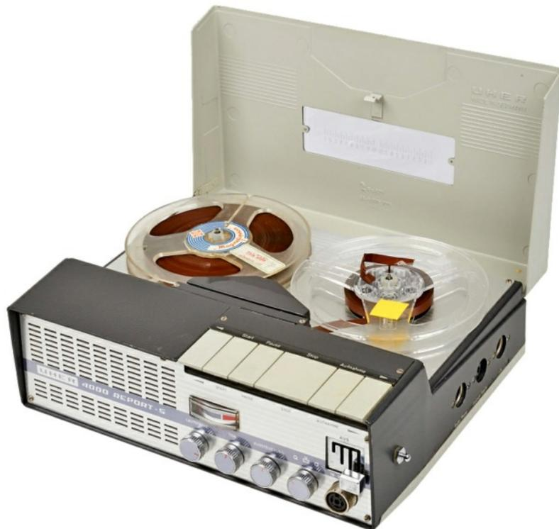
The Uher 4000 report-s, reel to reel, 2-track mono tape recorder was one in a series of high grade portable tape recorders. It was developed and manufactured by Uher in Munich, Germany, introduced in 1961. Photo courtesy Cryptomuseum, Holland.
